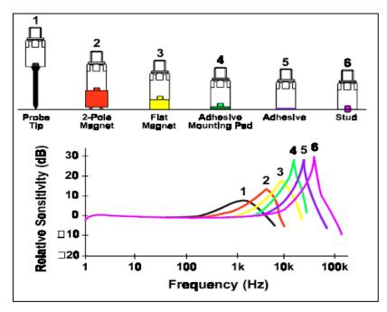
Different sensor mounting methods have different frequency responses. The onboard probe tip (#1 in diagram at left) will respond to vibration differently than the magnet mount external sensor (#2 in diagram at left). Both sensors can be used for machine screening with the 4-level severity scale and both sensors can be used to trend readings, as long as all of the trend measurements come from the same sensor type. Do not mix data from different sensor types into a single trend.
