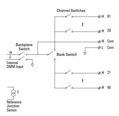
Note: Thermocouples must be electrically isolated from each other to avoid current loops and subsequent measurement errors.
