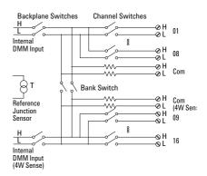
Note: Not recommended for connection to ac line without external transient suppression.
