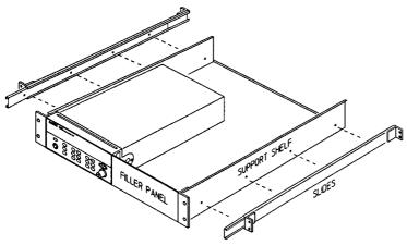
To install one or two instruments in a sliding support shelf, order shelf 5063-9255, and slide kit 1494-0015 (for single instrument, also order filler panel 5002-3999).
