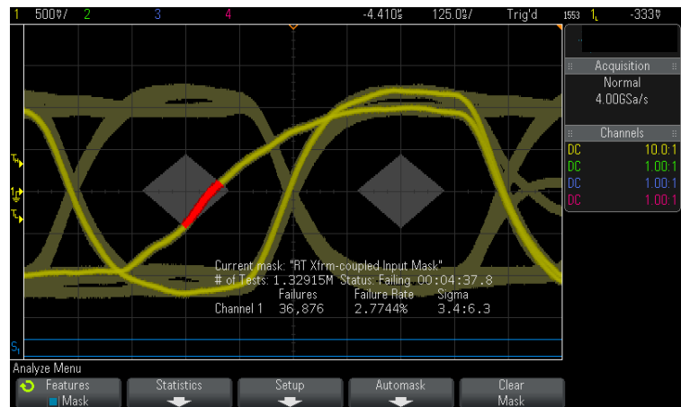
Figure 4. MIL-STD 1553 eye-diagram mask test.
