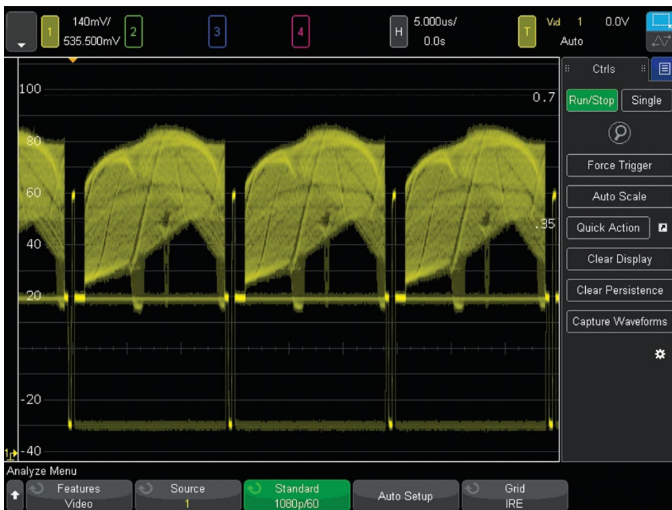
Figure 6. Triggering on 1080p HDTV.
