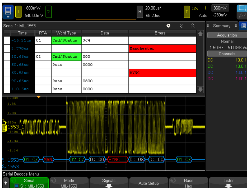
Figure 2. MIL-STD 1553 decode on an InfiniiVision X-Series oscilloscope.
