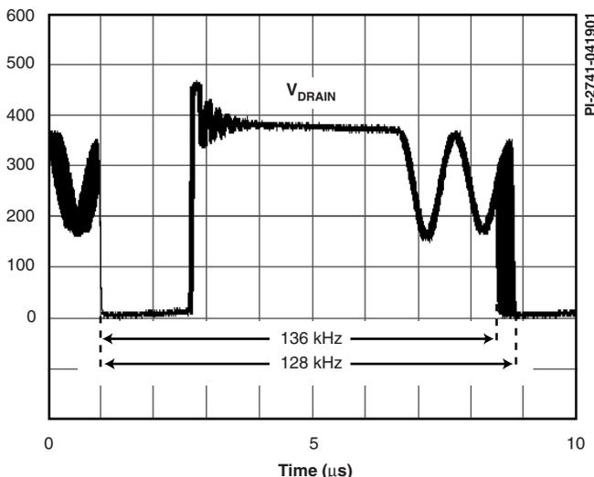
Figure 4. Frequency Jitter.
