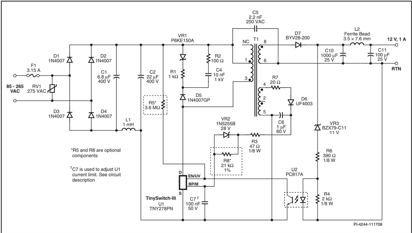
Figure 14. TNY278P, 12 V, 1 A Universal Input Power Supply.
