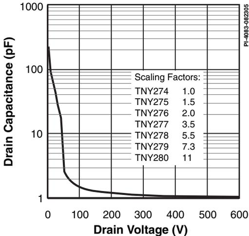
Figure 25. C<sub>oss</sub> vs. Drain Voltage.
