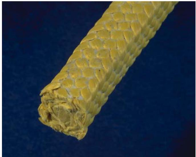
High strength aramid yarns with added PTFE as a break-in lubricant, Klingerlock braided to produce a packing for sealing within extreme pumping applications – rotary or reciprocating.
