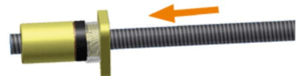
Press together the support nut 1. and the axial element 4. and thread the lead screw through the nut. Pre-tension the locking ring while doing so.
