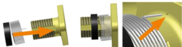
Position the friction disc 3. and the axial element 4. flush against the locking ring. Ensure that the locking ring does not rotate.
