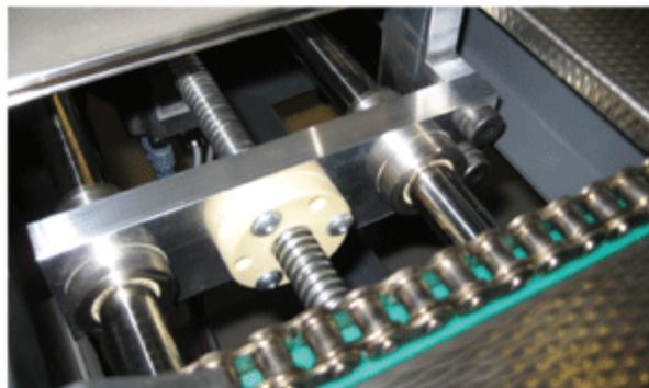
Format adjustment in the paper industry with anti-backlash lead screw nut
