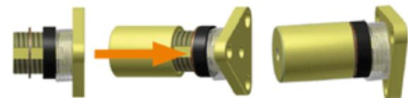
Thread the locking ring to the end of the support nut to tension the torsion spring.
