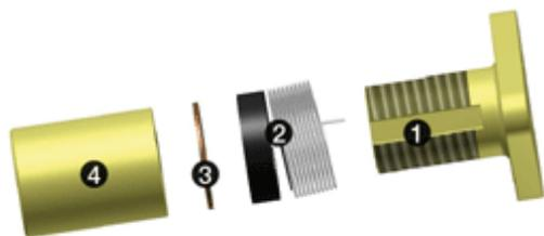
Thread the locking ring approx. half-way onto the support nut 1. using torsion spring 2., and secure the spring tab in the bore.
