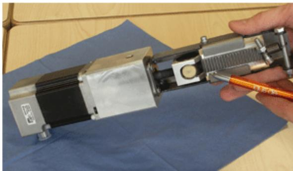
Anti-backlash lead screw nuts in a glue application system of a seam gluing machine (wood industry). These ensure the utmost in precision for the clearance-free adjustment mechanism.
