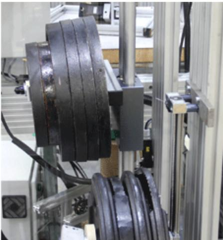
Test fixture at the igus® lab to determine service life
