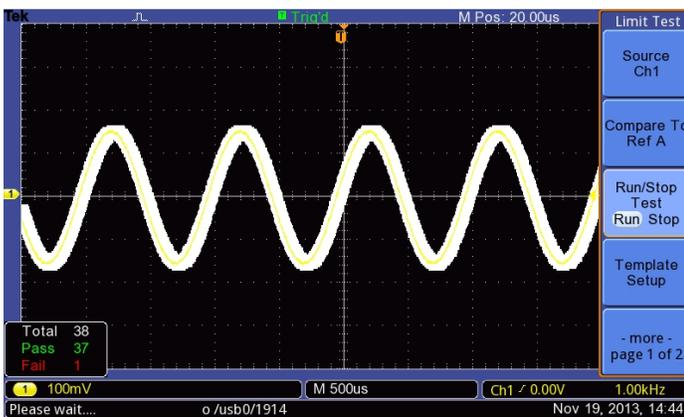
The Limit Test feature provides a quick Pass/Fail comparison between any triggered input signal and a user- defined template.
