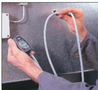
Measuring air flow with the Pitot tube
