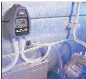
Measures flue draught, monitors filters and checks ventilators
